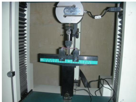
Fig 4: Specimen Loaded in Three Point Apparatus
