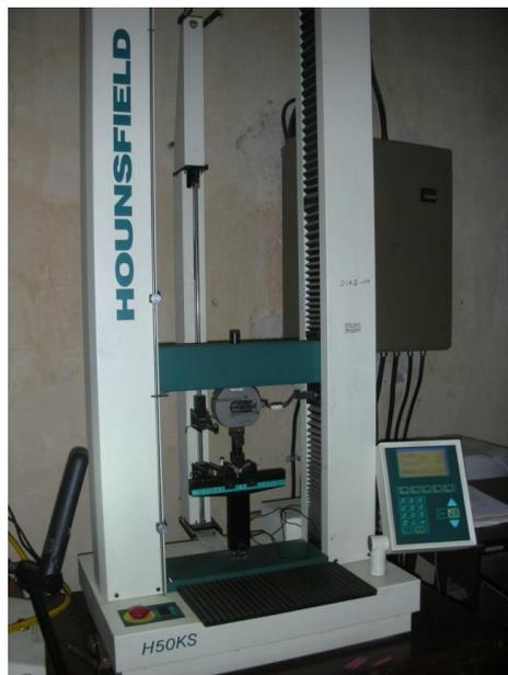
Fig 3: Universal Testing Machine
