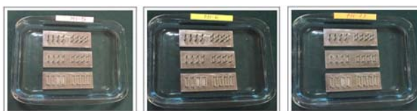
Fig 2: Glass Petridish with Stainless Steel Jigs Immersed In Saliva of PH 5, 6, 7.5 Respectively
