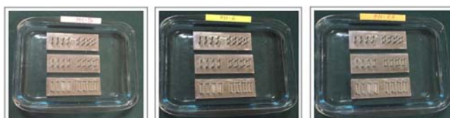
Fig 2: Glass Petridish with Stainless Steel Jigs Immersed In Saliva of PH 5, 6, 7.5 Respectively
