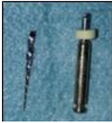
Fig 5: photograph showing a fractured ProTaper® (shaping file X) instrument. The instrument broke when inserted into the canal. We could speculate that it is a cyclic fatigue fracture by looking at the wear marks on the instrument's handle, adding that the instrument did not have time to be sheathed in the canal.
