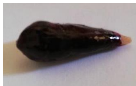
Fig 2: Painted the external root surface with two layers of nail polish except the most apical 2mm
