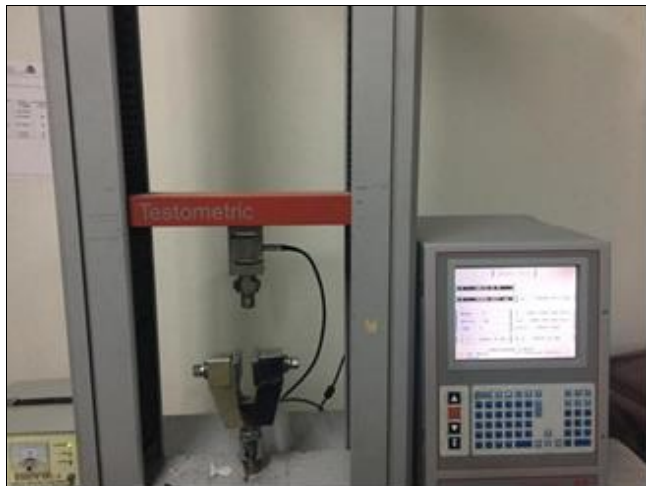
Fig 2: Universal Testing Machine (Test metric)
