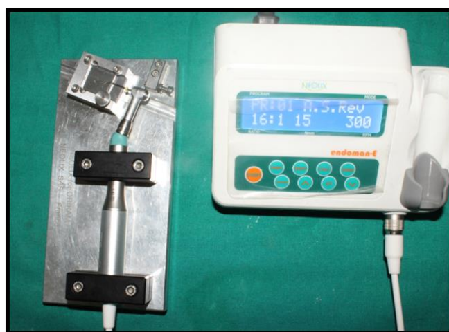
Custom made artificial groove simulating the root canal with curvature of 45 degree
