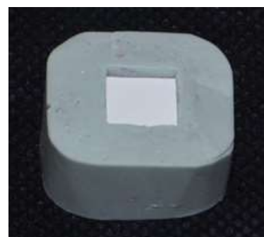
Fig 1: The mould for PEEK layering with composite
