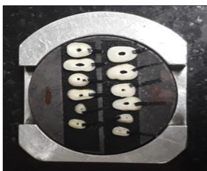
Fig 1b: EDS analysis on metallic stubs
