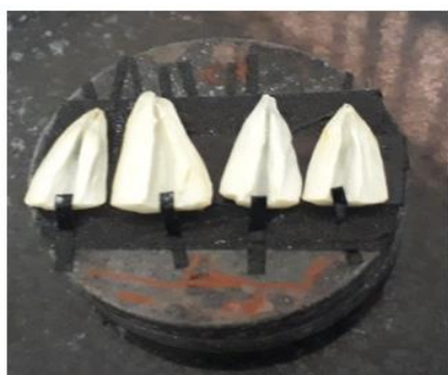
Fig 1a: Mounting of specimens for SEM
