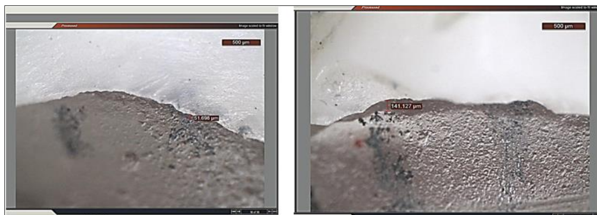
Fig 6: Measurement of marginal gap at two points marked on the epoxy die in conventional group
