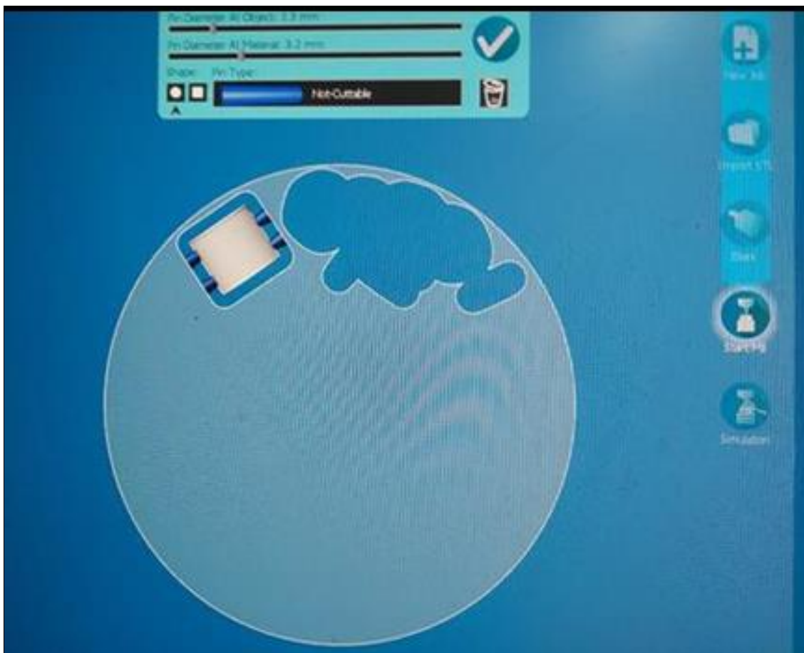
Fig 2: Cylinder nesting procedure inside zirconia disc on Exocad software
