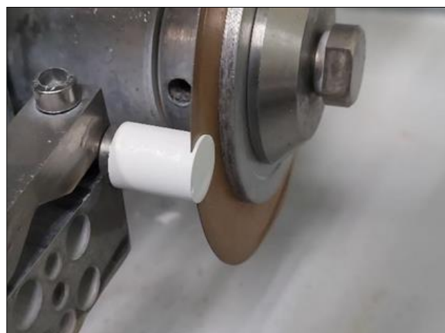
Fig 4: Sectioning of the zirconia cylinder with Isocut® Wafering Blades
