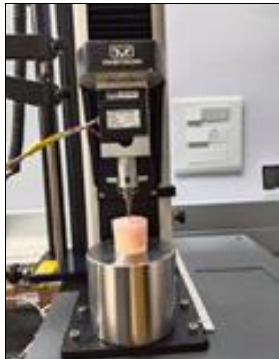
Fig 3: Testing of sample under Universal Testing Machine
