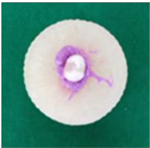
Fig 2: Sample mounted on acrylic block with addition silicone simulating periodontal ligament space
