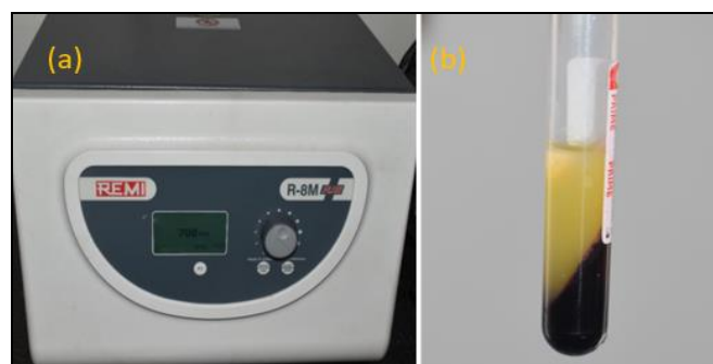
Fig 3: Preparation of platelet-rich fibrin (a) Digital Centrifuge machine at 2700 rpm for 12 min. (b) Obtained PRF clot
