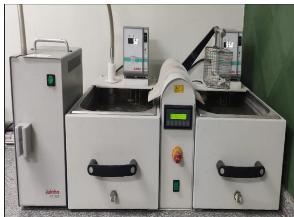
Fig 23: Thermocycler used for artificial ageing of specimens in this study.
