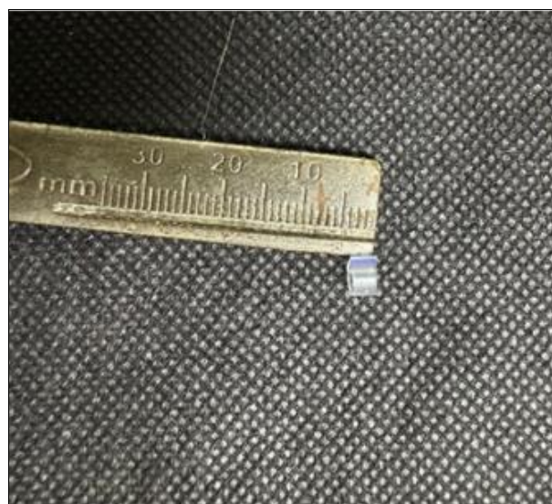
Fig 18: Silicone mold (Ryle’s tube) after cutting to the desired length
