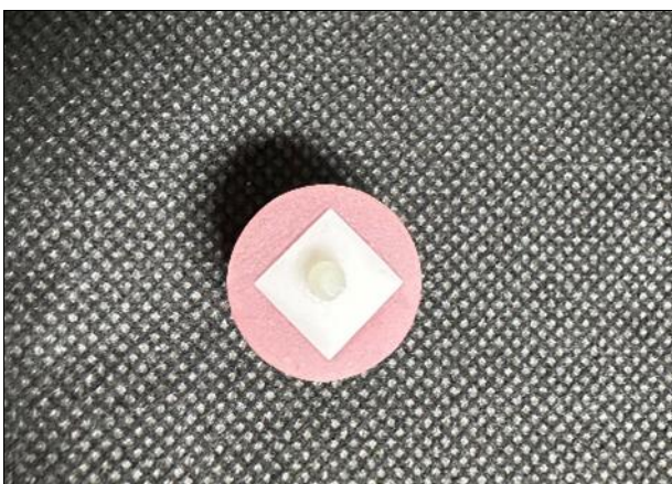
Fig 22: Specimen after resin cement bonding and removal of silicone mold
