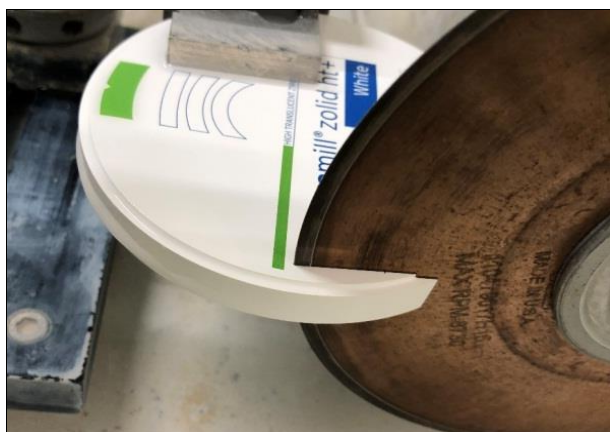
Fig 7: Sectioning of zirconia by Isomet
