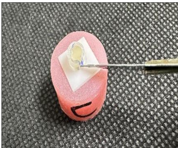
Fig 20: Scalpel blade number 11 used to remove silicone mold from around the resin cement
