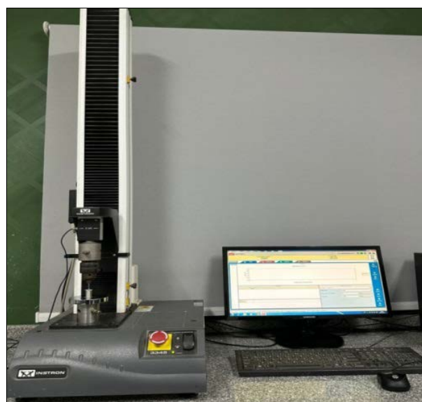
Fig 25: Instron testing machine model 3345 England
