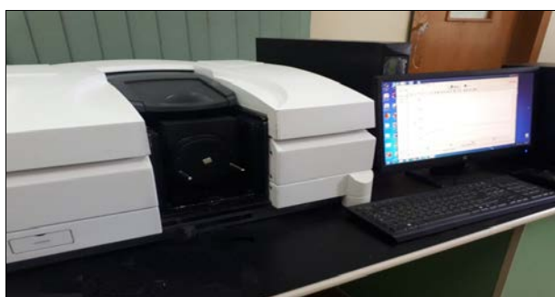
Fig 23: Agilent Cary 5000 spectrophotometer
