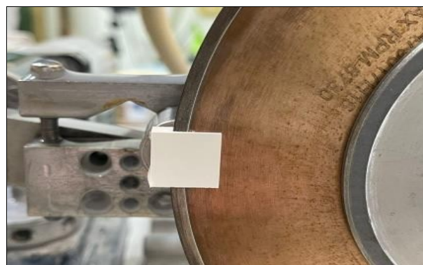
Fig 16: Isomet blade cutting IPS e.max zircad prime
