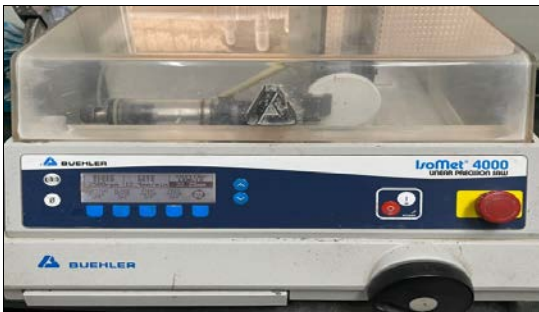
Fig 8: IsoMetM 4000 precision sawing machine
