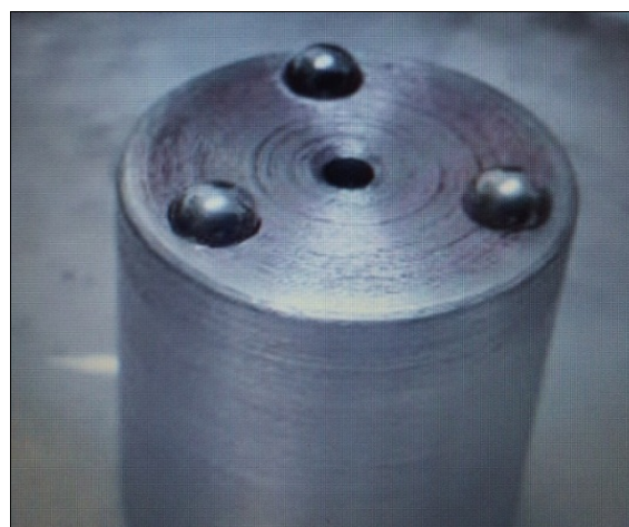
Fig 26: Metallic Platform with steel balls
