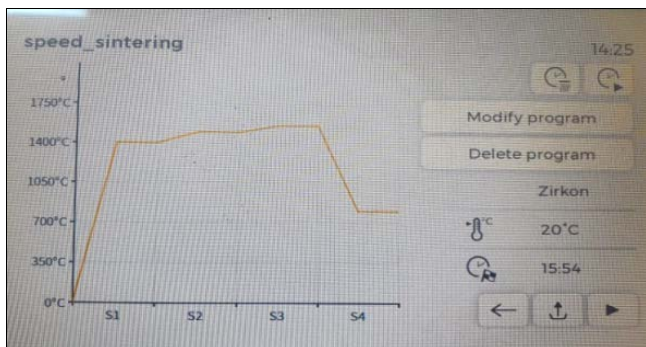
Fig 13: Dentsply's sirona inlab profire speed settings
