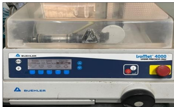
Fig 20: IsoMetM 4000 precision sawing machine
