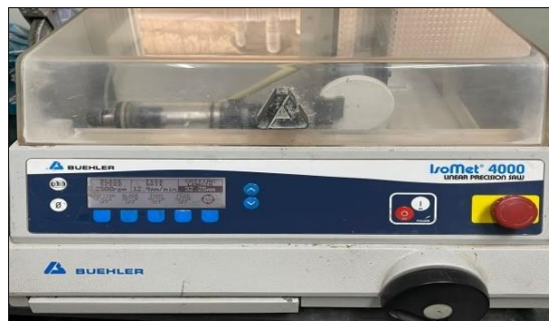
Fig 15: IsoMetM 4000 precision sawing machine
