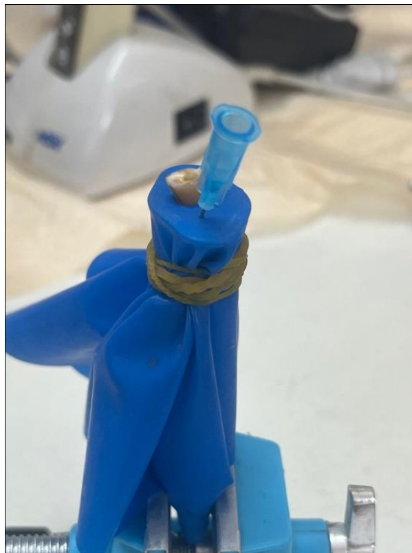
Fig 1: Coating the vial with rubber dam and insertion of ventilating needle through stopper and the root inside the rubber stopper.
