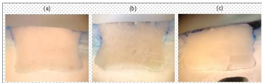
Fig 1: Marginal leakage in (a) Group-I (Fuji IX GP), (b) Group-II (AH Fil + ), and (c) Group-III (GI Ceramic Reinforced Extra)
