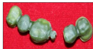
Fig 4: Castable resin pattern printed
