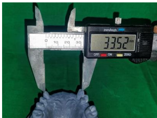
Fig 4: Measuring distance with digital vernier caliper on reference model
