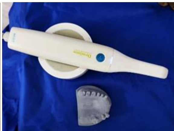
Fig 5: Reference model scanned using Rainbow scanner [Group A]
