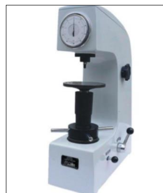
Fig 4: Each specimen were taken under Rockwell hardness testing machine
