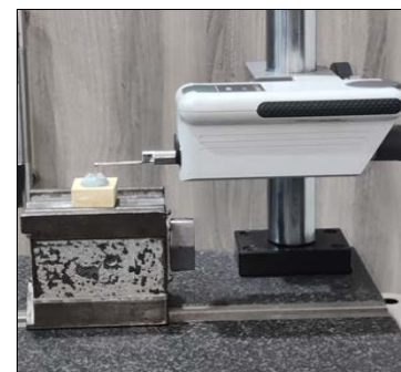
Fig 5: Surface roughness Tester
