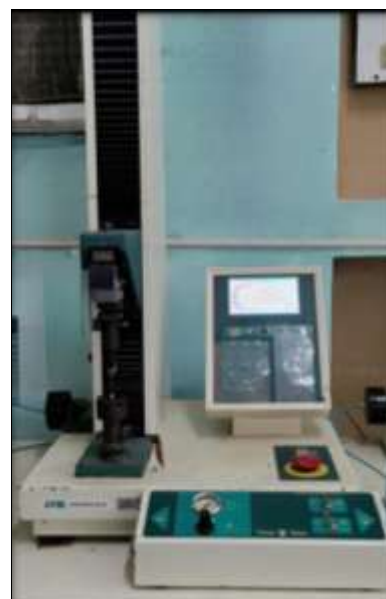
Fig 8: Universal testing machine, specimen subjected to microtensile bond test
