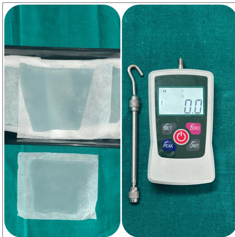
Fig 2: a) Light cure custom Tray material b) Force gauge - device displays the dislodging forces in newtons and registers the peak force
