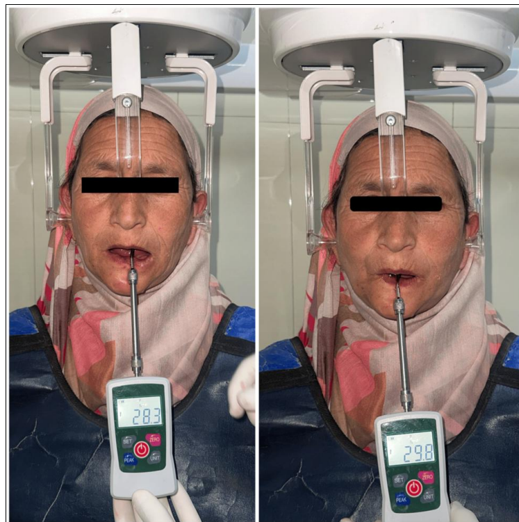
Fig 9: A digital force measurement gauge was used to record the retention of each maxillary denture base in the patient while maintaining the Frankfort horizontal (FH) plane parallel to the floor. Measurements were taken for two groups: (A) Green Stick Compound and (B) Light-Cure Material
