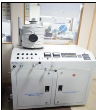
Fig 1: Electrostatic spray-assisted vapor deposition, Hindhi Vac, India
