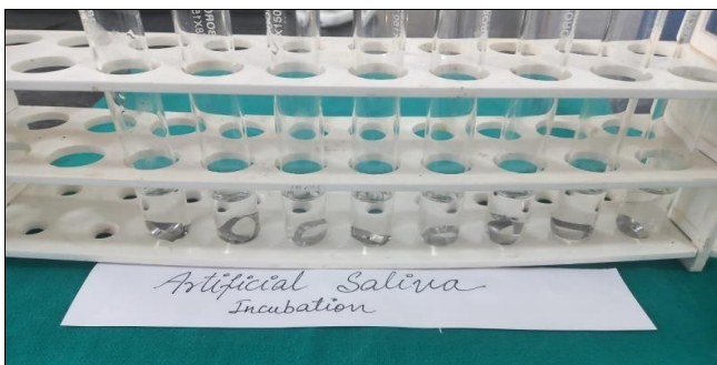
Fig 7: Incubation in artificial Saliva
