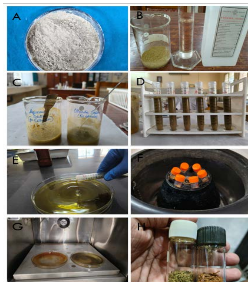
Fig 1: Extraction method. A - Eucalyptus powder, B - Water and ethanol tubes, C - Mixed with water and ethanol (99.9%), D - Poured into test tube, E- Centrifuged, F - Supernant collected into plates, G - Evaporated, H - Aqueous and ethanolic extracts.
