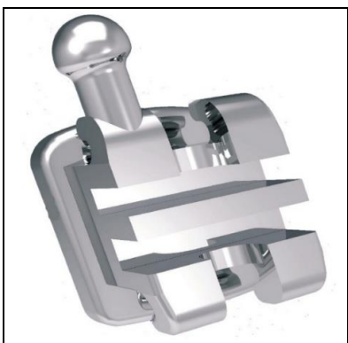
Fig 4: Kodan Duploslot (double slot) orthodontic bracket showing dual .018" and .022" slots. Image courtesy: KODEN ( https://kodenindia.com/dupslot-brackets.html )
