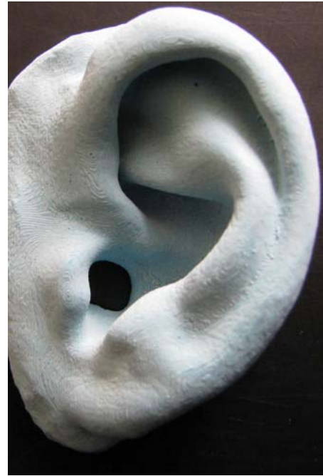
Fig 2: Thermoplastic prototype of the ear prosthesis made stereolithographically.
