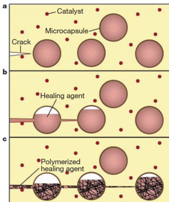
**Fig 4:** Basic method of the microcapsule approach (White *et al.*, 2001)
