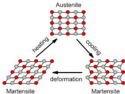
Fig 1: Nickel-Titanium Smart Alloy
