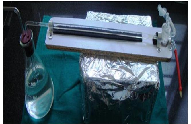
**Fig 13:** Fluid filtration model assembled for evaluation of apical microleakage
