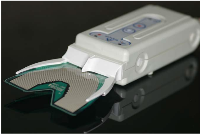
Fig 1: T-Scan III recording handle connects directly to a computer via a USB interface.
