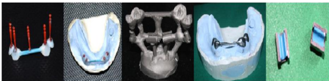
Fig 1.8: From left- Wax pattern was made, casted along with the metal housing for positioning clips, trimmed and polished, tried on the cast along with positioning clips with metal
