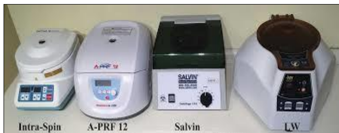
Fig 1: The four centrifuges used to produce L-PRF clots and tested in this study. From left to right: original L-PRF centrifuge
