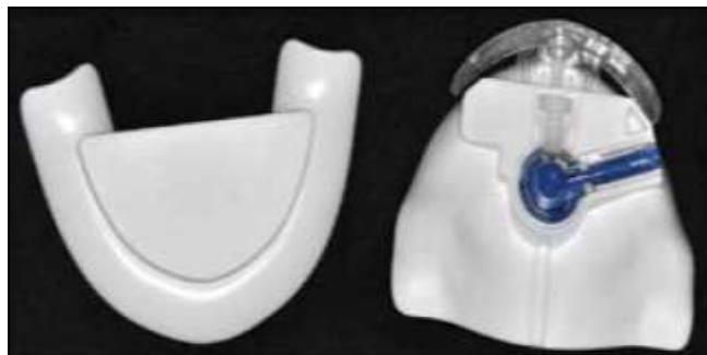
Fig 1: Maxillary and mandibular trays of the Anatomic Measuring Device (AMD)
