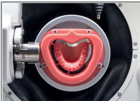
Fig 11: Wax bases fabricated with Ceramill Motion 2
