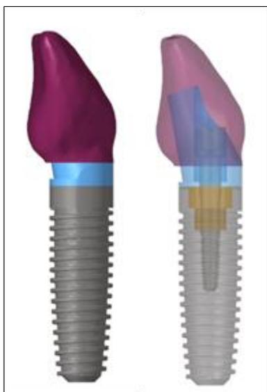
**Fig 2:** The CAD model images showing implant, screw, abutment and crown on abutment
