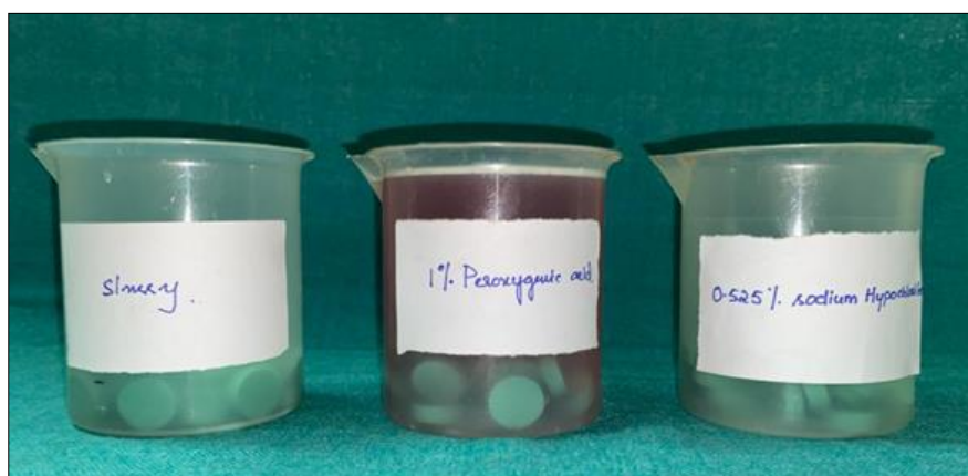
Fig 3: Immersion of specimens in Slurry, 0.525% Sodium Hypochlorite & 1% Peroxygenic Acid
