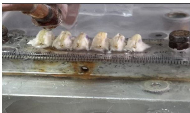
Fig 2: Specimens sectioned from the occluso-cervical dimension with a sectioning machine (Gillings-Hamco, Rochester, NY)
