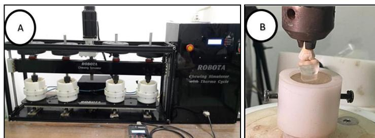
**Fig 3:** (A) The chewing simulator (ROBOTA) (B) the chewing simulator chamber with the enamel antagonist is in the upper compartment while the epoxy resin die in the lower compartment.
