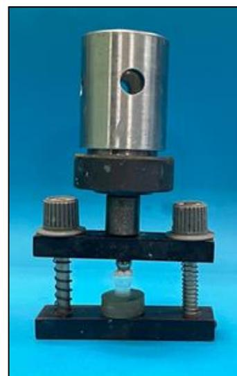
**Fig 2:** A customized loading device with a constant load of 3 Kg applied during occlusal veneers cementation to their corresponding epoxy resin dies.
