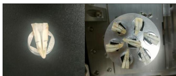
Fig 2: Specimens glued on metal stubs using electro-conductor glue and then transferred to ESEM plate
