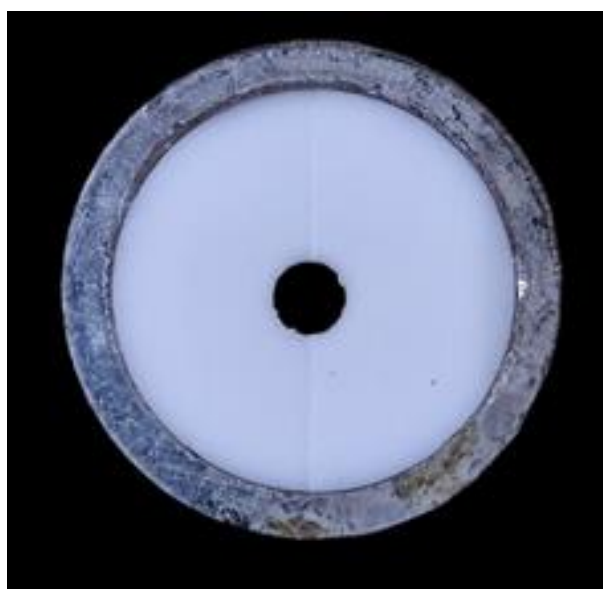
Fig 4: A customized split mold cylinder with an inner diameter of 3 mm and a height of 2 mm
