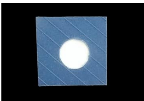
Fig 3: A customized blue tape with a central hole of 3 mm diameter on a PEEK sample
