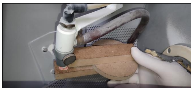
Fig 2: One of the arms of the wooden holder fits on the airblasting machine nozzle to adjust the angle of projection
