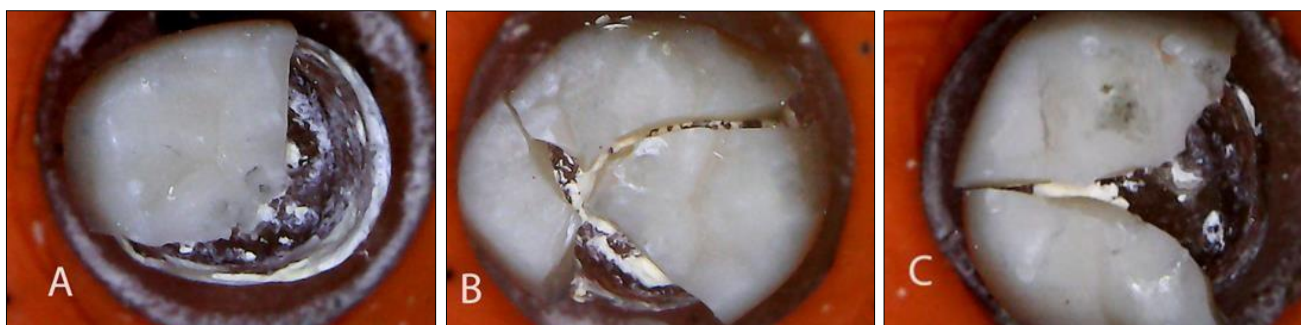
Fig 8: Digital microscope photograph (x25), mode of fracture of Oblique group (120°) (A) nonaged. (B) Thermocycling, (C) Thermo mechanical
