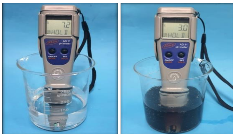
Fig 4: PH meter measure the PH of artificial saliva is 7.2, PH of cola beverage is 3
