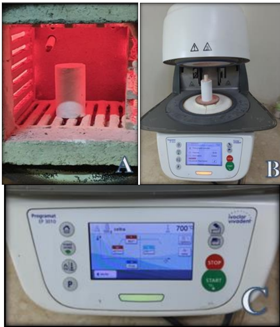
Fig 3: A: Placing the muffle in the furnace at 850 degree Celsius for 45 minute, B: Placing the entire assembly in Ceramic pressing Furnace, C: Adjusting the mode of furnace for Celtra press program
