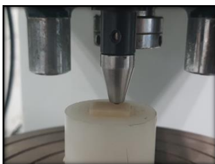
Fig 5: Vicker Tester with diamond indenter
