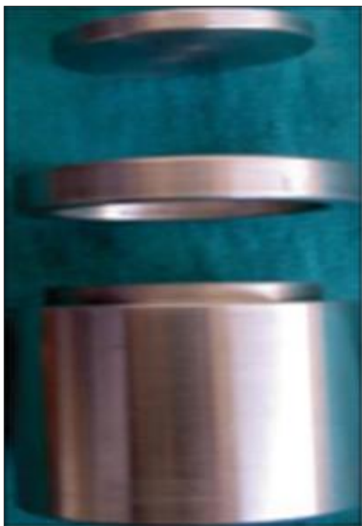
Fig 2: Components of ADA specification 19 stainless steel
