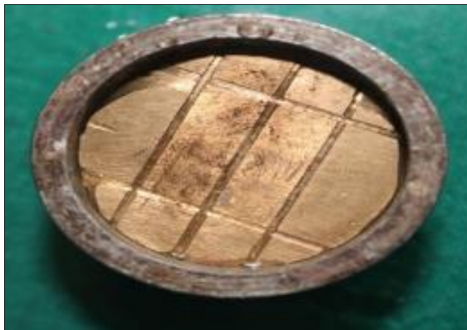
Fig 1: Lines inscribed on ADA specification 19 stainless steel die.
