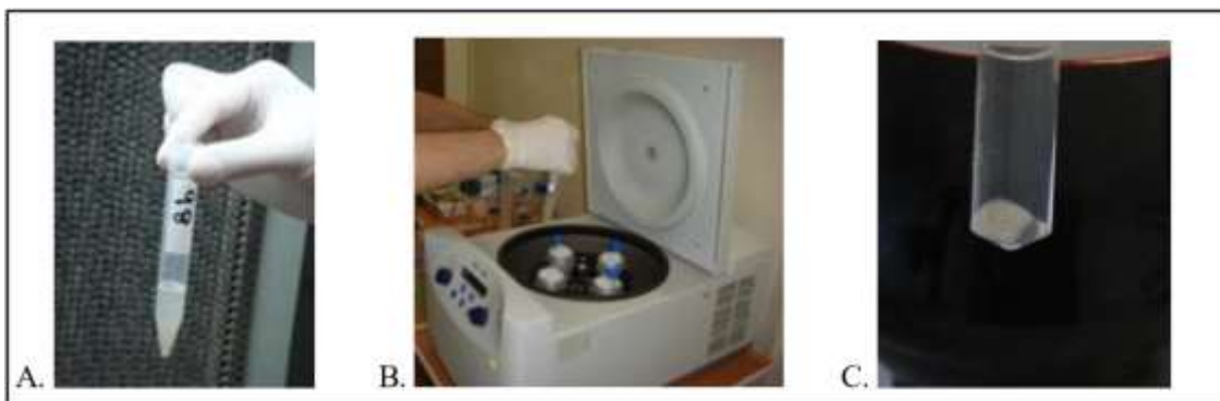
Fig 3: (A)-Samples placed in centrifuge tubes, (B)-The samples were subjected to centrifugation at 3000 rpm for a duration of 10 minutes, (C) Saliva after centrifugation
