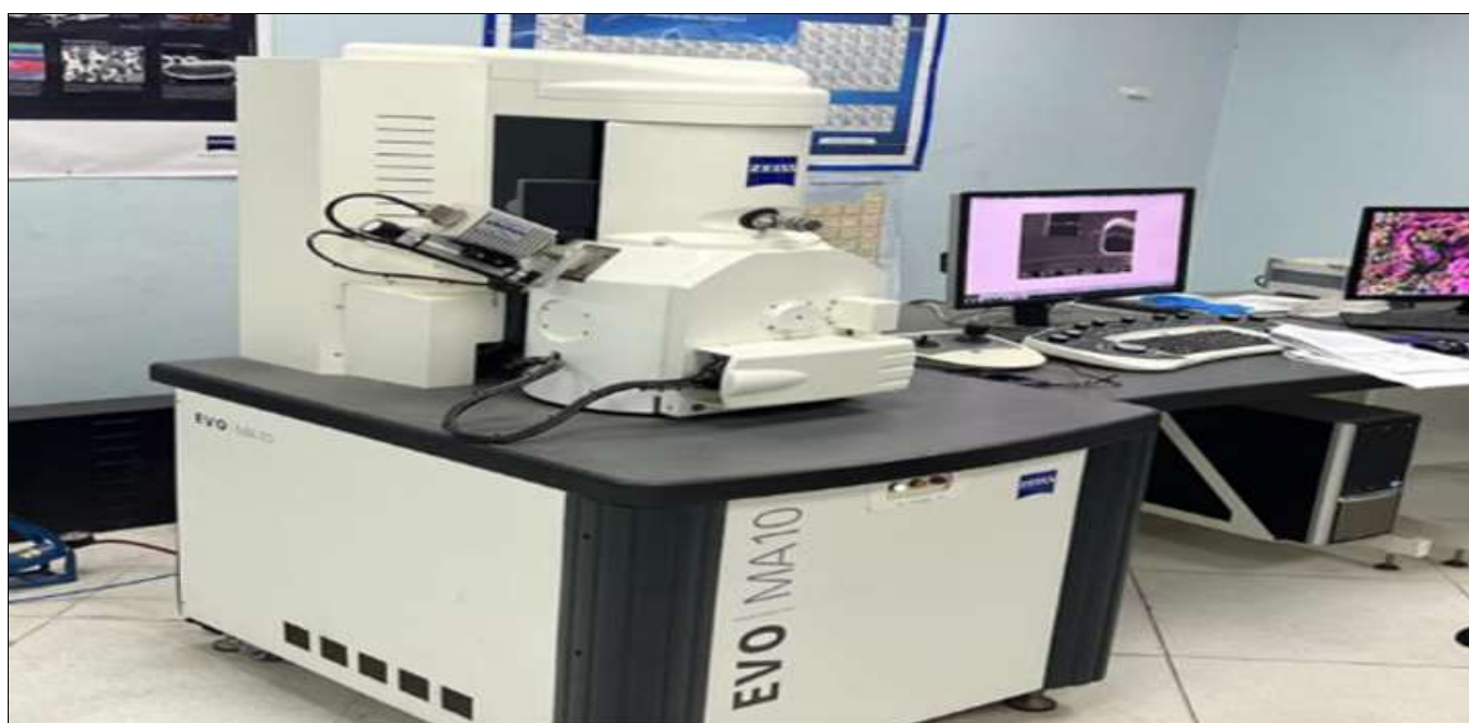
Fig 1: Scanning Electron Microscope (SEM) model (Zeiss EVO MA10)
