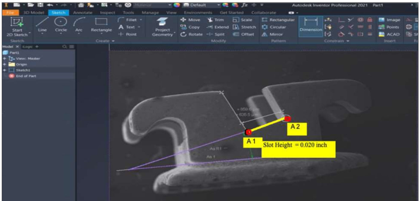
Fig 2: An image from Autodesk inventor software showing a lateral view of upper left central incisor (Dentaurum) measuring the slot height with the two reference points A1 and A2
